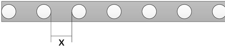
Figure 2: Schematic diagram of an NIR air nozzle bar; nozzle spacing ranges from 12.5 mm to 37.5 mm
